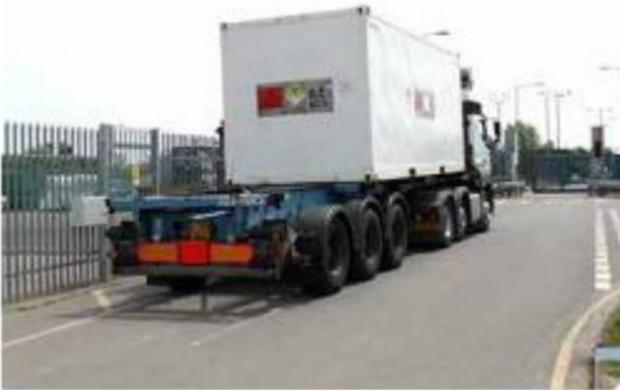
FED which has experienced a longer period of radioactive decay (ie older) and is therefore lower in activity has already been transferred from Bradwell to Dungeness A in an industrial package. This transfer has
