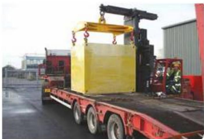
Magnox ILW will be packaged into containers suitable for final disposal. The ductile cast iron containers (DCICs) to be used at Bradwell, Berkeley, Dungeness A, Hinkley Point A, Oldbury and Sizewell A are also transport containers. Type VI containers are an example of an industrial package. Mosaik<sup>®</sup> containers can be either industrial packages or Type B packages.
